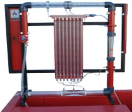
flow meter demonstration
