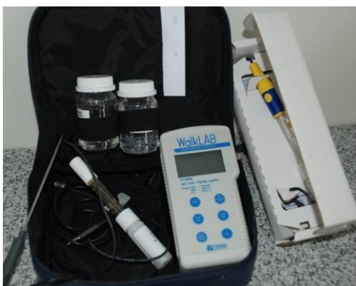
Ph meter difital battery opp-spear electrode
