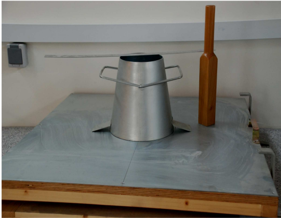
Apparatus for Determinate flow in concrete(flow table)
