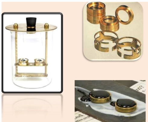
ring and ball apparatus for softening point of bitumen
