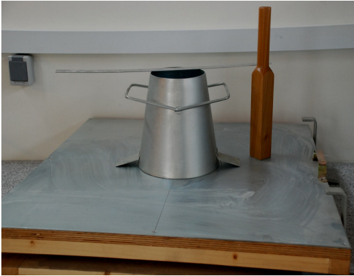
Apparatus for Determinate flow in concrete(flow table)
